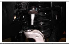
Separate the upper control arm from the steering knuckle using an 18mm socket. Note: the upper control arm will be under tension.
