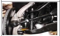
Reinstall the sway bar end links using a 13mm socket for the bottom.
