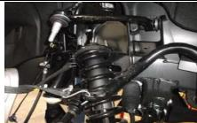
Lift the sway bar out of the way, then remove the strut from vehicle.
