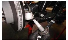
Remove the tie rod ends from the steering knuckle using a 21mm socket. Note: You may need to use a hammer to separate the ball joint from the knuckle.
