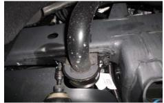
Loosen the factory sway bar at the frame using a 10mm socket.
