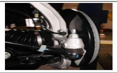
Reinstall the tie rods into the knuckle using a 21mm and 10mm wrench.
