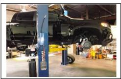
Lift the vehicle by the frame. Then remove the front wheels using a 22mm socket.
