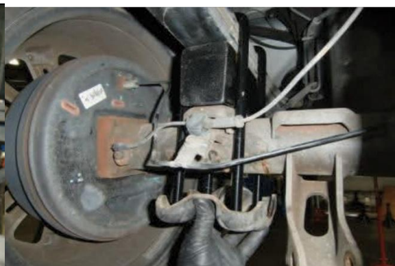
Reinstall lower plate.
