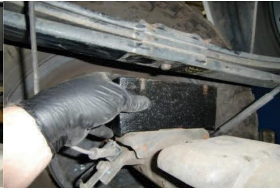
Tapered Blocks: Place block and take care that the pin is aligned with the hole in the block.
