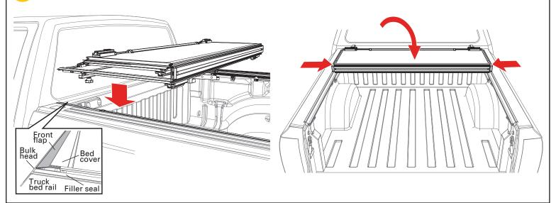
Rotate the cover retainer clamp (G) installed earlier so that it is aligned with its long side going side to side with the truck. The tabs of the cover retainer clamp (G) will align with the diagonal arm of the bed brace as shown. Align the retainer clamps on both sides and tighten the knobs by turning them clockwise until the lock washer is secure. Repeat on the driver's side.
