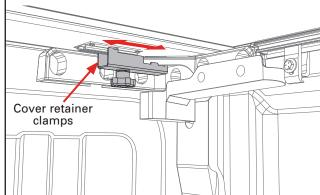
The retainer needs to be in the side to side orientation, do not angle the position.
