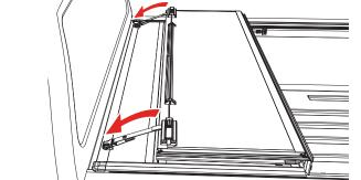
FLIPPED UP POSITION: Fold the cover (A) open and lift it until it's vertical or past 90 degrees towards the truck cab. Then release the prop rod that is attached to the rail. Fold the prop rod over and position it firmly against the vertical plate on the underside of the cover. Then slide the prop rod locks downwards and tighten the knobs to lock it into position. Do this on both sides of the cover. The cover should be firmly in position with little to no movement once the prop rods are locked.
