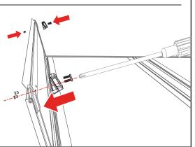
Before placing the cover (A) onto the vehicle, slide two cover retainer clamps (G) into the track on the underside of the cover (A) near the cab. Confirm the cover retainer clamps fit properly into the cover rail for optimum fit. Repeat on the opposite side of the cover.
