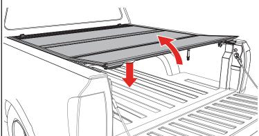
**FOLDED UP POSITION:** To drive with the cover (A) in the folded up position, use the straps and buckles provided with the cover. Attach the buckle at the bulkhead, then pull the strap to take up the slack and secure the cover.
