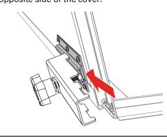
Set the cover (A) in the folded position on the side rails (B) & (C) towards the cab of the truck. Make sure the front flap is on top of the truck bulkhead. Confirm the cover is evenly spaced between the rails.
