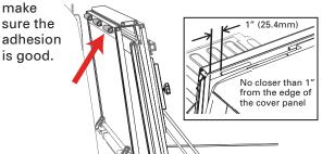
Unfold the cover (A) towards the tailgate. Then confirm each panel is centered side to side and front to back on the truck bed. If adjustments are needed, loosen the cover retainer clamps (G) and shift the cover until positioned correctly. The rear edge of the cover and tailgate seal should rest on top of the tailgate. For proper sealing, the tail panel will overlap by .5".
