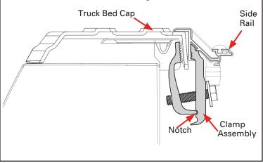
Place the outer part of the stake pocket clamp (U) into the stake pocket, up underneath the plastic bed cap, then secure to the bolt. Make sure the rail is level. Tighten all clamps to 10 ft/lbs of torque with a 1/2" wrench or socket. Caution: Do NOT overtighten! Note: For 07-13 models only, install stake pocket covers (V) into stake pocket opening in the side rail toward tail. Repeat for driver's side rail (B).
