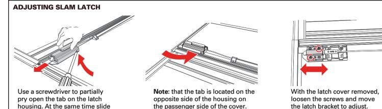
loosen the screws and move the latch bracket to adjust. Retighten the screws. Slide the latch housing back on.
