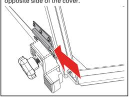
For the best (A) fit, the side rails (B & C) should be level with the truck bed cap and not angled up or down. Insert the backside of the clamp as high as possible and tighten clamp. Depending on model the notch will vary. Tighten all clamps to 10 ft/lbs of torque with a 1/2" wrench or socket. **Caution: Do NOT overtighten!**
