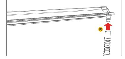
Place the driver side rail (B) on the truck rail. Position the side rail flush with the top edge of your truck bed rail. The end of the side rail with the drain tube will go towards the cab of the truck. Repeat on the opposite side with the passenger side rail (C).
