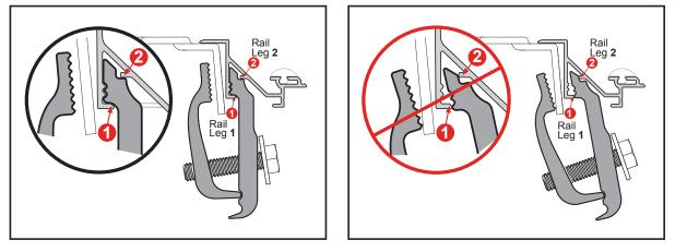
**Water Intrusion:** Make sure the retaining clamps are tight and properly engaged to the side rails. Check that the bulkhead seal is in place and the cover is resting on it. Make sure that all latches are engaged to the side rails and adjust if needed. Check that the side rails are installed flush with the top of the bed rail.
