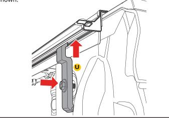
Before placing the cover (A) onto the vehicle, slide two cover retainer clamps (G) into the track on the underside of the cover (A) near the cab. Confirm the cover retainer clamps fit properly into the cover rail for optimum fit. Repeat on the opposite side of the cover.
