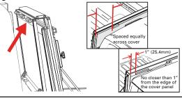
**18** Unfold the cover (A) towards the tailgate. Then confirm each panel is centered side to side and front to back on the truck bed. If adjustments are needed, loosen the cover retainer clamps (G) and shift the cover until positioned correctly. The rear edge of the cover and tailgate seal should rest on top of the tailgate. For proper sealing, the tail panel will overlap by .5".
