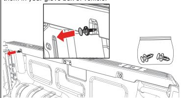
Install the brackets (E), bolts (C) and nuts (D) provided using a 30 Torx bit on passenger and driver side bed caps where you removed the two corner clips in step 1. Make sure the nut is behind the sheet metal.
