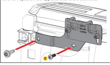
7 Tighten the Torx screw removed in step 4 using a T-45 Torx bit and torque to 16ft-lbs (22Nm) & using a T-30 Torx bit and torque screw (C) to 8ft-lbs (11Nm). Repeat on the opposite side of the truck bed.
