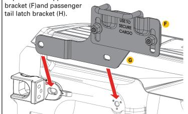
Re-install one of the T-45 Torx screws from step 8 through the bracket (G) and into the same hole you removed it from. Then install one of the provided T-30 Torx screws (C) into the other hole in the same bracket and into the hole in the side of the bed. Loosely fasten the screws. Repeat on the opposite side of the truck bed.
