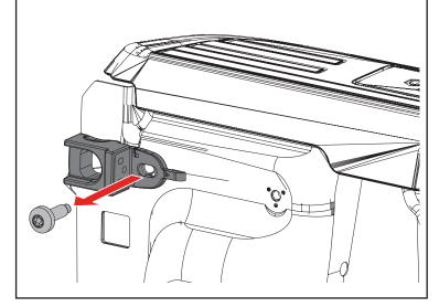
The brackets are assemblies comprised of the striker bracket (F) and a driver tail latch bracket (G). Align the two holes in the driver tail latch bracket (G) with the tailgate slam bumper hole you removed the Torx screw from in step 8 and the other hole in the side of the bed as shown. Repeat on the opposite side of the truck bed with striker bracket (F) and passenger
