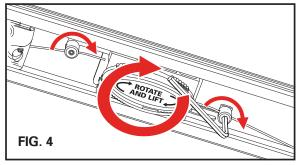
Double-check that the cover is secure and tight to the truck bed by gently lifting the corners to ensure the mechanisms are engaged. To make the final adjustment, loosen the striker bracket nuts. Then move the striker bracket (F) down by firmly pushing the cover (A) or pulling the rear bow downward to the truck rail and tailgate. Make sure that both sides match, then retighten the screws.
