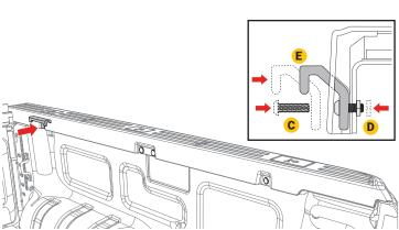
Remove the T-45 Torx screw from the tailgate slam bumper. **Do not discard screw**. Repeat on the opposite side of the truck bed.
