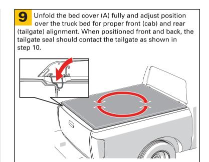
Close the tailgate and unfold the cover. Check that the cover is parallel and square with the truck bed and bed rails. Adjust the cover until the bulb seal fits with the tailgate as shown. If not parallel or square, open the cover and loosen the cab clamps to reposition the cover. If the cover is too far back the tailgate will not close.
