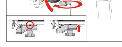
Unfold the cover (A) towards the tailgate. Then confirm each panel is centered side to side and front to back on the truck bed. If adjustments are needed, loosen the cover retainer clamps (G) and shift the cover (A) until positioned correctly. Retighten the cover retainer clamps once the desired fitment is reached. If adjustments to the slam latch are needed, see the directions on the next page.
