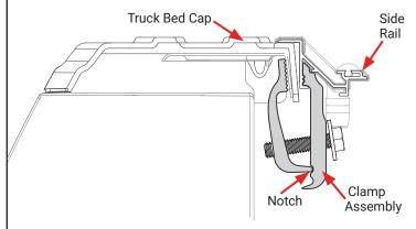
7 Attach one stake pocket clamp (J) from the passenger side rail (A) to the truck bed. Disassemble the stake pocket clamp (J). Place the inner part of the clamp into the rail. Make sure the bolt passes through the stake pocket hole as shown.
