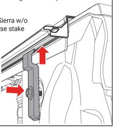
**9** Before placing the cover (C) onto the vehicle, slide two front cover retainer clamps (F) into the track on the underside of the cover (C) near the cab. Confirm the cover retainer clamps fit properly into the cover rail for optimum fit. Repeat on the opposite side of the cover.
