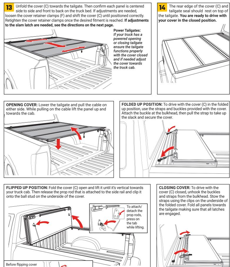
(C) in the up position make sure to stow the straps using the clips on the underside of the folded cover.
