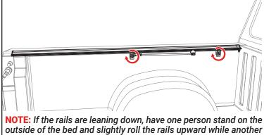
outside of the bed and slightly roll the rails upward while another person slowly snugs the clamps up. If the clamps are tightened too quickly or overtightened, it will cause the rails to lean down. 4 Place the passenger side rail (A) on the truck rail. Position the side rail flush with the top edge of your truck bed rail. The end of the side rail with the drain tube will go towards the cab of the truck. Repeat on the opposite side with the driver's side rail (B).
