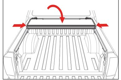
Place the outer part of the stake pocket clamp (J) into the stake pocket, up underneath the plastic bed cap, then secure to the bolt. Make sure the rail is level. Tighten all clamps to 10 ft/lbs of torque with a 1/2" wrench or socket. **Caution: Do NOT overtighten!** Install stake pocket covers (K) into stake pocket opening in the side rail toward cab and tail. **Repeat steps 5-8 on the opposite side with the driver's side rail (B)**.
