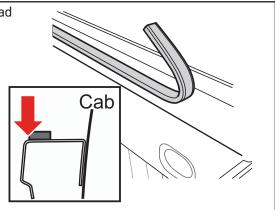
2 If rubber filler strips (E) were **NOT** included in your kit, skip to step 3. If you received rubber filler strips (E) with the cover (C), clean the rail the same way as you did in step 1. Peel the backing and adhere the filler strips (E), as illustrated, between the truck plastic bed cap and truck metal rail. Place one 6-8 inches from the bulkhead. Place the rear strip as close to the tailgate as possible. Center the middle strip appropriately.
