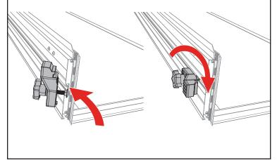
Position the buckle ends (I) with the open side facing the bed cover panel. Use a screwdriver to install the two buckles into the pre-drilled holes on the front header panel with the provided screws (J). DO NOT use a screw gun, securely tighten by hand only.
