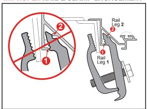
**Water Intrusion:** Make sure front retaining clamps are tight and properly engaged to the side rails. Check that the bulkhead seal is in place and the cover is resting on it. Make sure that all latches are engaged to the side rails and adjust if needed. Check that the side rails are installed flush with the top of the bed rail.
