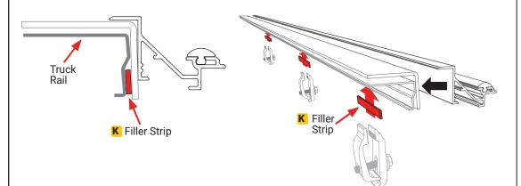
IMPORTANT: In order for the cover (A) to operate properly the side rails (B & C) MUST be square (90° angle) to the truck bed rails. This allows the rear latch to engage properly.
