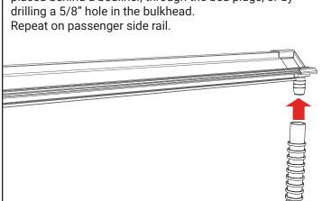
Place the driver side rail (B) on the truck rail. Position the side rail flush with the top edge of your truck bed rail. The end of the side rail with the drain tube will go towards the cab of the truck. Repeat on the opposite side with the passenger side rail (C).
