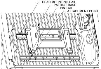
Figure C3: View into truckbed looking back at tailgate. Copyright 2016, B&W Custom Truck Beds, Inc. ALL RIGHTS RESERVED **3. IMPORTANT:** Before drilling forward mounting holes pull the RV base towards the rear of the truck and push the forward rail towards the cab of the truck to correctly space the mounting rails, see figure C4.
