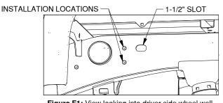
Figure F1: View looking into driver side wheel well.
