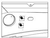
**3a.** Install the front side plates (without overload brackets). Locate the two front side plates, four 1/2" lock washers, four 1/2" finish nuts. Pass the top flange of the rear side plates over the frame and then pass the holes in the side plates over the carriage bolts. Secure the side plates with a 1/2" lock washer and nut, see Figure F4. Hand tighten hardware only at this time.
