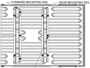
DRILL LOCATIONS HIGHLIGHTED \_/Figure A2: Detail view over bed, showing drill BY BLACK DOTS locations for the forward and rear bed rails.
