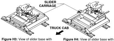
Figure H3: View of slider base with the carriage in a foward position. TOWING POSITION
