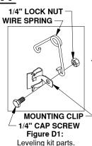
2. Attach kit. Locate the flange which will be closest to the truck cab on the driver side pivot arm, see Figure D2. The clip should be placed so that when the spring's coil is in the line with the edge of the arm there will be 1/2" of clearance between the bottom of the polyurethane bushing and the top of the spring, see Figure D3. Drive the clip securely onto the flange with a hammer.
