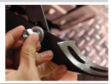
For 2017 diesel models only: Trim DEF tank shield as needed and reinstall.
