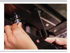
Bolt the def-tank support bracket to the back of the def-tank L-bracket using a M10 hex bolt, flat washer and lock washer.
