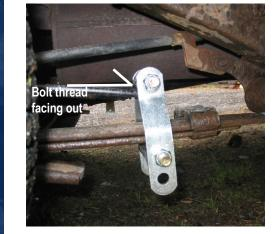
Front Use upper bolt hole position on the front shackle to ensure frame clearance.
