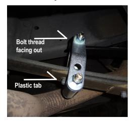
Front Use upper bolt hole position on the front shackle to ensure frame clearance.
