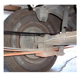
SuperSprings are installed on top of axle.
