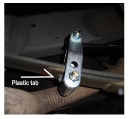
Rear Install the shackle against the axle side of the last plastic tab.
