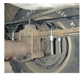
SuperSprings are installed on top of MTKT mounting kit.
