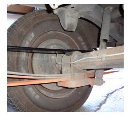
SuperSprings are installed on top of axle.
