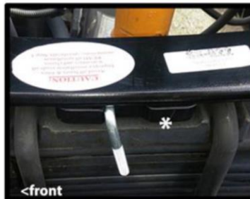
Place PSP11 on top of spring plate flat side up facing, with groove toward the front
