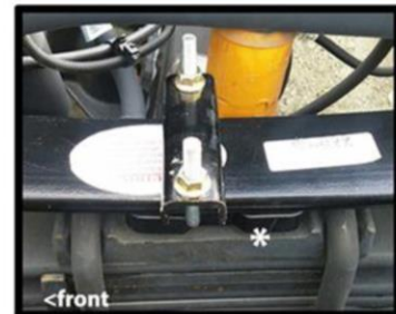
Install the SuperSprings as pictured below, then thread the channel crossplate on to the bolt. Tighten securely.
