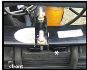
Install the SuperSprings as pictured below, then thread the channel crossplate on to the bolt. Tighten securely.
