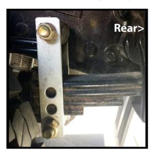
\*Where chassis are equipped with top helper leaf the overload perches need to be unbolted and removed \*
