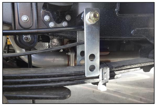
**Step 6:** Using a heavy duty C-Clamp or SuperSprings installation tool, pull down the rear shackle. Attach rear shackle with bolt, sleeve and roller (as in #5 above) and tighten. Don't over-tighten nuts. NEVER TIGHTEN TOP BOLTS ON ANY OF THE SHACKLES.
