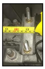
Step 4: Position the shackle on the front of the SuperSpring so that it is directly behind the sway bar link. (see picture at right). Ensure head of upper shackle bolt is clear of sway bar link!
