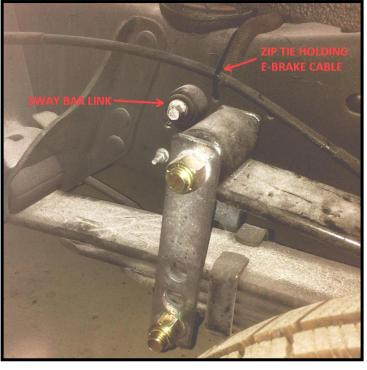
**Step 6:** Using a heavy duty C-Clamp or SuperSprings installation tool, pull down the rear shackle. Attach rear shackle with bolt, sleeve and roller (as in #4 above) and tighten. NEVER TIGHTEN TOP BOLTS ON ANY OF THE SHACKLES. (see picture below)
