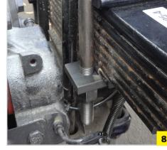
Fasten lower cross plate – Place a Clamp Plate (ITEM F) over the ends of the u-bolt and slide up to contact the bottom of the leaf pack. Place one 3/4" Flat Washer (ITEM G) and one 3/4" Nut (ITEM H) over each leg of the u-bolt and tighten until snug.
