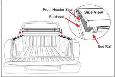
To connect the cover assembly (C) to the side rails (A and B), slide the right and left header guides into the locked position. A clicking sound will indicate a secure attachment.
