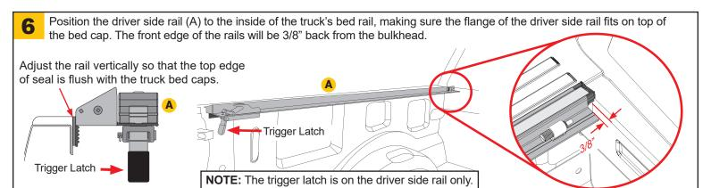
For optimal latching performance and cover fit, the side rails (A & B) should be level with the truck bed caps and not tilted up or down. To fine-tune side rail tilt, you can reposition the clamps (D). To adjust the rail tilt upwards or downwards. Tighten all clamps (D) with a T-30 drive socket or T-handle wrench.
