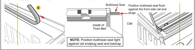
Place the cover (C) on the side rails towards the front of the truck bed (near the cab). The front header seal is designed to help shed water and should sit on top of the bulkhead.
