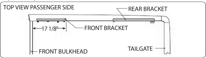
Adjust the lock strikes up or down accordingly. With the tailgate down adjust the lock strike to allow approximately 1/8" (3mm) play in the cover up and down.
