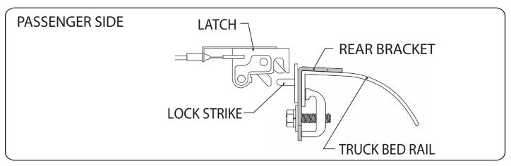
It may be necessary to adjust the latch side to side, to do so loosen the two latch mounting bolts, adjust latch and tighten.
