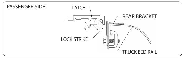
It may be necessary to adjust the latch side to side, to do so loosen the two latch mounting bolts, adjust latch and tighten.
