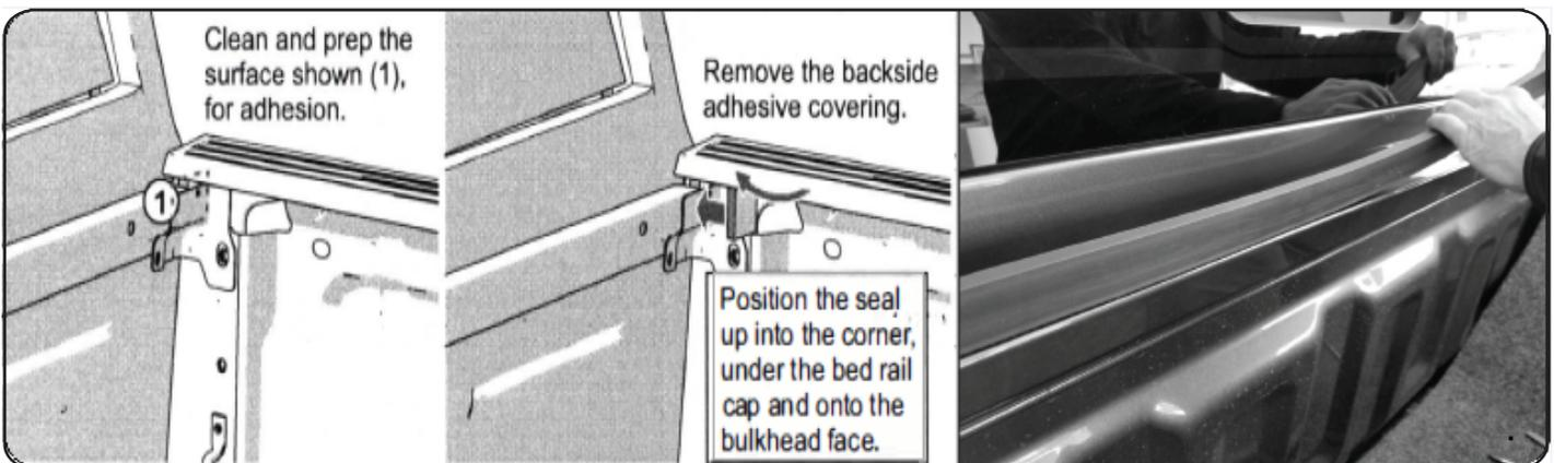
**Install the bulkhead weather seal to the truck's front bulkhead. After installing the bulkhead seals proceed to mounting the truck specific brackets.**
