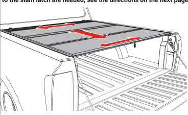
Power Tailgates: If your truck has a powered opening or closing tailgate ensure the tailgate functions properly with the cover closed and if needed adjust the cover towards the truck cab.
