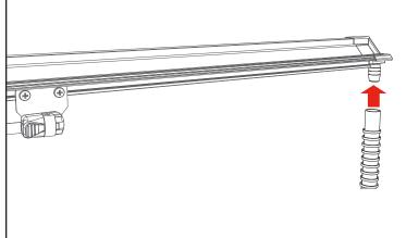
Place the passenger side rail (A) on the truck rail. Position the side rail flush with the top edge of your truck bed rail. The end of the side rail with the drain tube will go towards the cab of the truck. Repeat on the opposite side with the driver's side rail (B).
