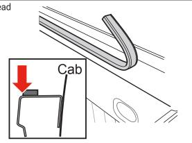
If rubber filler strips (E) were **NOT** included in your kit, skip to step 3. If you received rubber filler strips (E) with the cover (C), clean the rail the same way as you did in step 1. Peel the backing and adhere the filler strips (E), as illustrated, between the truck plastic bed cap and truck metal rail. Place one 6-8 inches from the bulkhead. Place the rear strip as close to the tailgate as possible. Center the middle strip appropriately.
