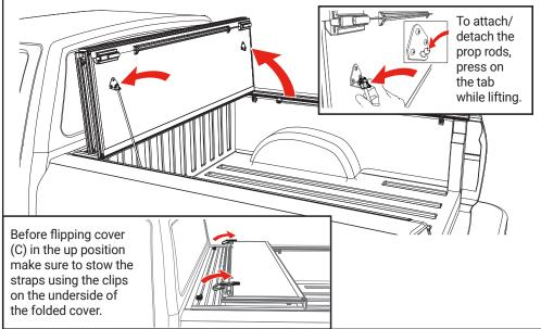
**CLOSING COVER:** To drive with the cover (C) closed, unhook the buckles and straps from the bulkhead. Stow the straps using the clips on the underside of the folded cover. Fold all panels towards the tailgate making sure that all latches are engaged.
