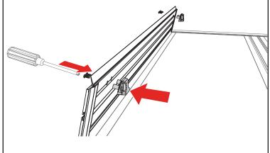
**12** Confirm the retainer clamps (F) are positioned around the side rails (A & B) correctly as shown below. Tighten the retainer clamps by turning them clockwise until the lock washer is secure
