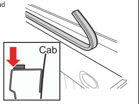
2 If rubber filler strips (E) were **NOT** included in your kit, skip to step 3. If you received rubber filler strips (E) with the cover (C), clean the rail the same way as you did in step 1. Peel the backing and adhere the filler strips (E), as illustrated, between the truck plastic bed cap and truck metal rail. Place one 6-8 inches from the bulkhead. Place the rear strip as close to the tailgate as possible. Center the middle strip appropriately.
