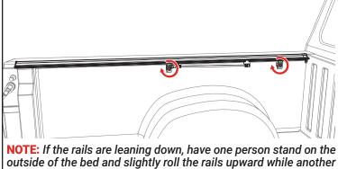
outside of the bed and slightly roll the rails upward while another person slowly snugs the clamps up. If the clamps are tightened too quickly or overtightened, it will cause the rails to lean down. 4 Place the passenger side rail (A) on the truck rail. Position the side rail flush with the top edge of your truck bed rail. The end of the side rail with the drain tube will go towards the cab of the truck. Repeat on the opposite side with the driver's side rail (B).
