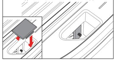
**10** Position the buckle ends (H) with the open side facing the bed cover panel. Use a Phillips screwdriver to install the two buckles into the pre-drilled holes on the front header panel with the provided screws (I). **DO NOT use a screw gun, securely tighten by hand only.**
