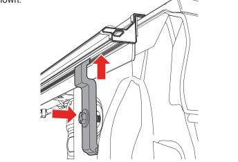
**9** Before placing the cover (C) onto the vehicle, slide two front cover retainer clamps (F) into the track on the underside of the cover (C) near the cab. Confirm the cover retainer clamps fit properly into the cover rail for optimum fit. Repeat on the opposite side of the cover.
