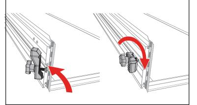
Set the cover (C) in the folded position on the side rails (A & B) towards the cab of the truck. Confirm the cover is evenly spaced between the rails.
