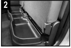
Position the Under Seat Storage under the backseat as shown.
