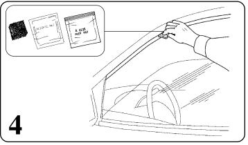
**STEP 5:** To install the front visor, remove the tape liner from the rear end flange. To reduce the risk of tape contamination due to improper positioning, expose only 2" (5cm) of tape from each end of the lateral flange by peeling back liner. See **FIGURE 5**
