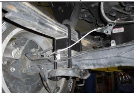
Attach lower mounting plate with provided hardware.
