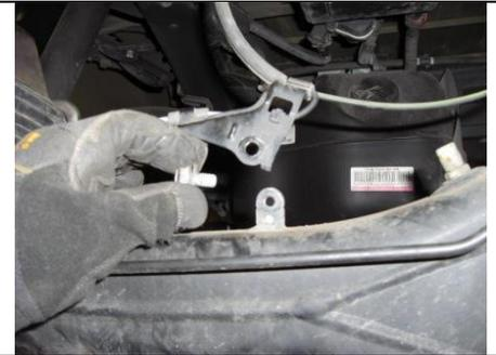
Disconnect ABS wiring brackets from axle.
