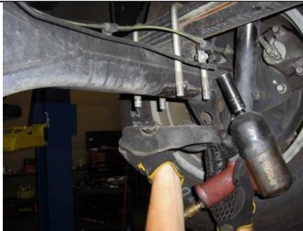
Remove u-bolt nuts and lower plate.
