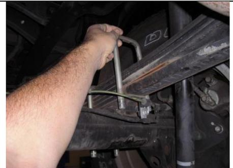
Carefully lower axle and remove u-bolts
