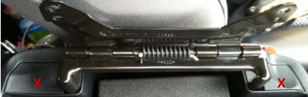
Red X's mark plastic covers that must be removed to access hinge screws.
