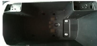
Place the Lock'er Down Console Safe inside the console and attach to the truck body through the console with the supplied longer bolts.
