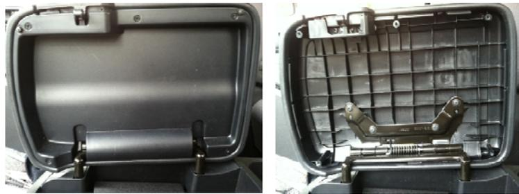
On either end of the hinge is a plastic cover that must be removed next. You can use a small screw driver or even a finger nail. Detailed photos on back.
