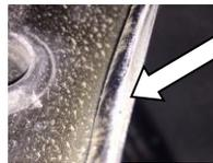
**Note:** Inner sealant bead in wheel well.
