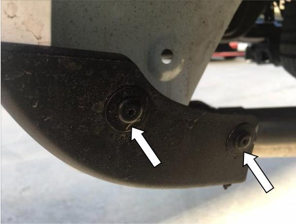
**STEP 14:** Using #15 Torx head screwdriver remove the two bottom screws from the rear factory spat. Maintain screws for re-install.
