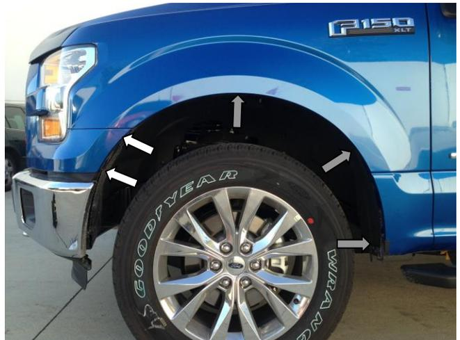
**STEP 6:** Locate three (3) 5.5mm bolts and two (2) 7mm bolt.
