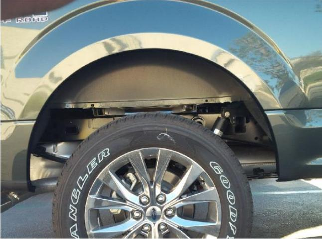
**STEP 15:** Clean the body areas where the Fender Flares will make contact. Use the supplied alcohol wipe.
