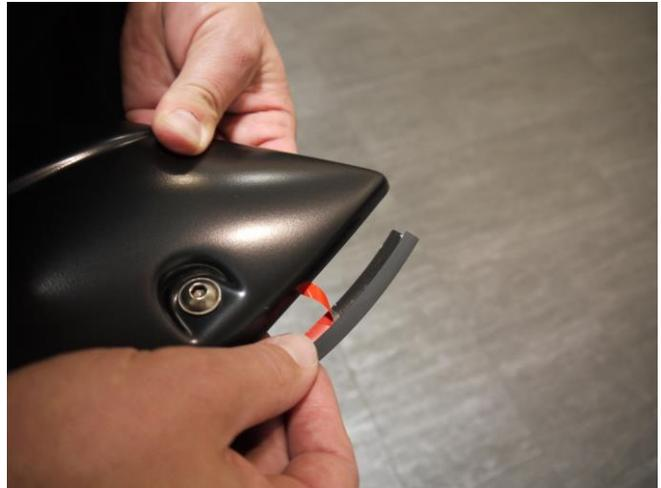
**STEP 12:** Attach the included rubber seal to the Fender Flares. Peel back 2" of the adhesive backing and position on the Fender Flare. Attach the seal to the Fender Flare, peeling back a few inches at a time. Attach rubber seal along all areas the Fender Flare will make contact with the vehicle body.
