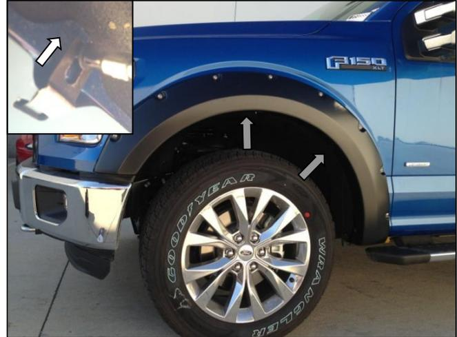
**STEP 8:** Place the Fender Flare onto the vehicle and fit into the correct position following the contours of the body. Use 2 of the retaining clips and 5.5mm bolts to secure the Fender Flare to the body. Make sure the clip securely engages the Fender Flare.
