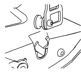
When the BEDXTENDER is at the furthest rear position, push down on the buckle to insert into tailgate latch. Tighten straps. To release, pull tailgate handle.
