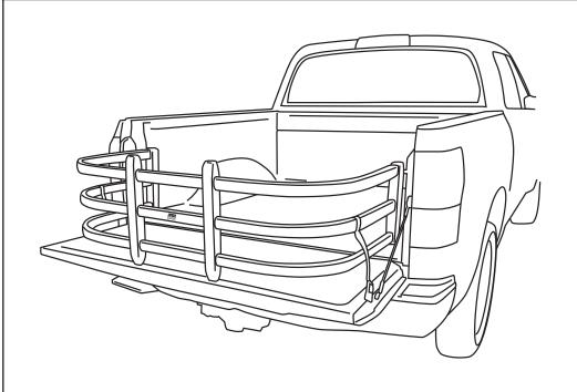
BEDXTENDER HD<sup>™</sup> shown assembled and installed on truck.
