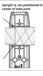
NOTE: The inside of the upright is stepped to fit correctly around the small and large diameter tubes. Tighten PT-Screws using a T-25 torx driver, starting in the middle of each upright, then the outer screws and lastly the remaining two to evenly tighten.
