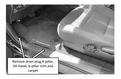
**Step 14:** On the DRIVER side, remove the front kick panel, front door sill trim panel and b-pillar trim panel. Go under the driver seat and locate the split in the carpet. Pull the rear half of the carpet back to expose the oval rubber drain plug. Pull the drain plug and drill a 7/16" hole.
