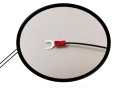
**Step 17:** The door trigger sensor harness will need a ground connection to the vehicle. Locate the seat belt assembly at the driver side b-pillar and install the ground wire under the top bolt of the seat belt assembly.
