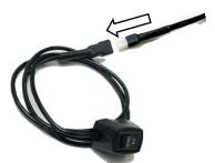
**Step 23:** Locate the black wires for the disable switch and feed them to your desired mount location. Prepare the surface by cleaning with a 50/50 mix of isopropyl alcohol and water or equivalent. Once the surface is dry, peel the backing from the double-sided tape and stick the disable switch on the lower dash panel. Plug the disable switch connector into the black wire harness and tuck the extra wire behind the lower dash panel.
