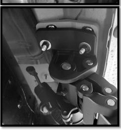
**Step 4**: Install the FRONT DRIVER side motor using (2) M8 flat washers, (2) M8 lock washers and (2) M8 hex nuts, to fasten the motor to the bracket. The hardware should be hand tightened only until snug. This will allow the motor assembly to move and align easier when installing the running board.
