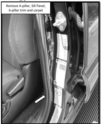
**Step 16:** Route the DRIVER side door trigger wire (brown) towards the DRIVER side b-pillar. Route the PASSENGER side door trigger wire (white) and the black disable switch wires under the center console to the left side of the vehicle. The white wire needs to go to the passenger side b-pillar, the black wires will go to the center console.
