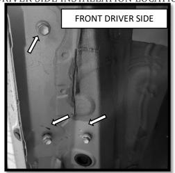
**Step 3**: Locate and remove the 3 factory bolts. Place in the inner part of the front driver bracket (2) M8x30mm Hex bolts, threads must be pointing out. Install the FRONT DRIVER bracket using (3) M8X30mm Hex Bolts, with (2) M8 flat and lock washers to fasten the bracket to the vehicle. NOTE: The outer corner bolt must not have washers.
