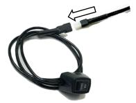
**Step 23:** Locate the black wires for the disable switch and feed them to your desired mount location. Prepare the surface by cleaning with a 50/50 mix of isopropyl alcohol and water or equivalent. Once the surface is dry, peel the backing from the double-sided tape and stick the disable switch on the lower dash panel. Plug the disable switch connector into the black wire harness and tuck the extra wire behind the lower dash panel.
