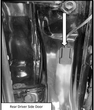
**Step 20: REAR DOOR** Apply a vertically oriented strip of masking tape on the rear Driver side door using the door stopper as a reference point. Make a mark 3.5" below the center line of the latch. Prepare the surface by cleaning with a 50/50 mix of isopropyl alcohol and water or equivalent. Once the surface is completely dry, peel the backing from the double-sided tape and stick the magnet to the door. Align the top of the magnet with the 3.5" mark as shown.
