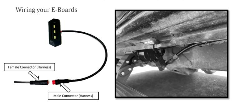
**Step 12**: Align the arrows on the small round connectors and plug the Driver side front and Driver side rear LED lights. Prepare the surface by cleaning with a 50/50 mix of isopropyl alcohol and water or equivalent. Once the surface is completely dry, peel the backing from the double-sided tape and stick the LEDs to the bottom side of the rocker panel. Position the LED lights at the center of the front and rear passenger side doors
