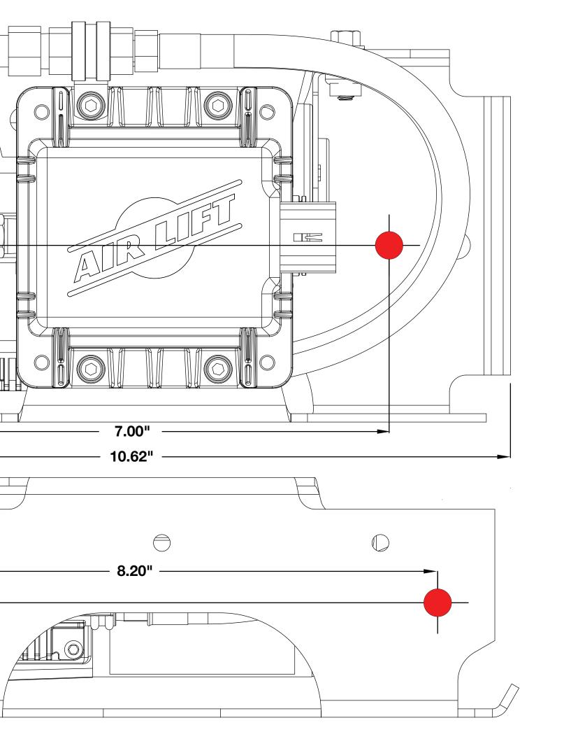
5. Connect the wiring harness (C) to the manifold (Fig. 2). Press the connector on completely and listen for an audible "click." Press white lock on connector toward manifold to lock connector in place. Ensure a proper drip loop exists to prevent water intrusion (Fig. 6). Install the fuse (E) last. The system will automatically fill to 5 PSI (.34BAR) once the fuse is installed.
