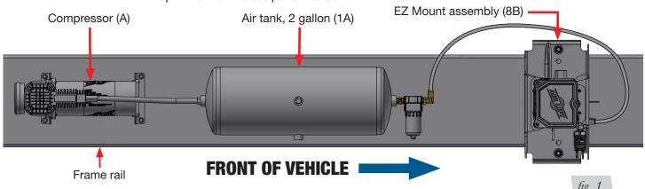
Avoid routing air lines and wiring near sharp edges. If passing air lines or wiring through holes in the frame, use rubber grommets (not supplied) (Fig. 2). Support wiring and air lines every 8-12" (200-300mm) with zip ties or other means.
