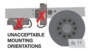
holes if using self-tapping screws. If mounting from the frame, before drilling, ensure that the back side of the frame is clear of vehicle components, including brake lines, fuel lines, wiring, etc. Do not remove components from the EZ Mount assembly.
