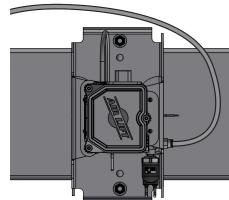
2. EZ Mount can be mounted in any orientation except with the electrical connector pointed down or with the Air Lift logo facing the ground (Fig. 11). There are mounting holes in the web of the EZ Mount bracket and in the top flange. Use the included drilling template (Figs. 21 & 22) for mounting with self-threading screws or hex cap bolts. Use a 1/4" drill bit to make pilot
