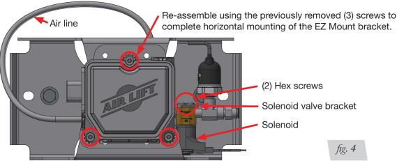
5. Remove the (2) hex screws from the solenoid valve bracket/assembly (Fig. 4) using a 3/32" hex wrench.
