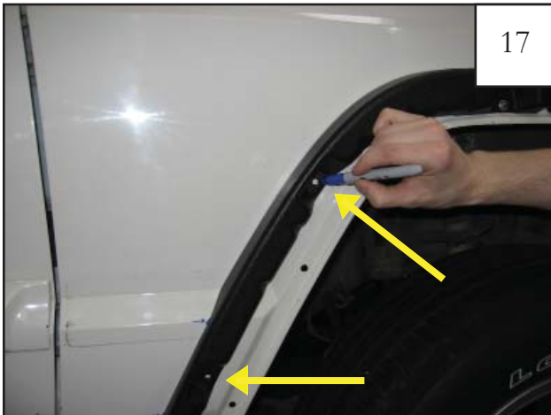
Align outer edge of inner piece P2 (D2 for driver side) with the measuring lines made in Step 14. Use a grease pencil or marker to mark the rear hole locations on the sheet metal.
