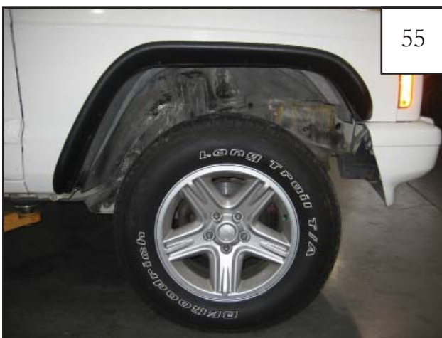
Completed front passenger's side flare installation.
