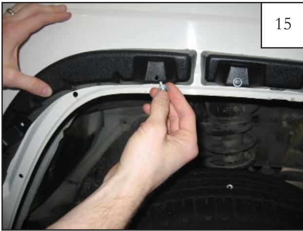
Position inner piece P2 (D2 for driver side) on fender, aligning upper hole with the existing factory hole in sheet metal.
