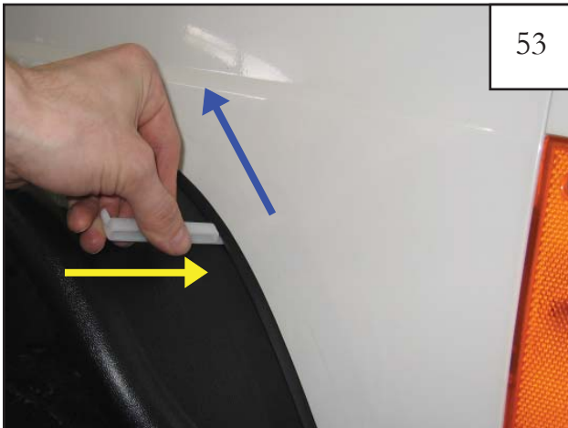
Starting at one end, place the flat edge of the supplied edge trim tool between the lip of the edge trim and the surface of the flare then slide along the edge trim while pressing it in toward the vehicle surface to further ensure proper adhesion.
