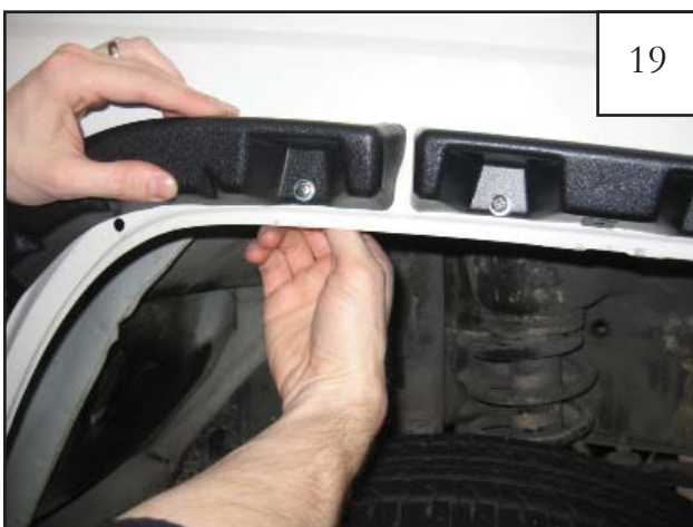
Reinstall inner piece P2 (D2 for driver side) by aligning the part with the upper factory hole and newly drilled holes. Attach inner piece to the sheet metal with a screw/washer and flange nut in each hole location. Only hand tighten at this time.
