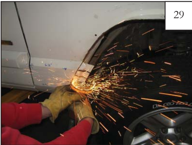
Use cut off saw to cut along horizontal lines. Do not cut past profile line made in step 22.
