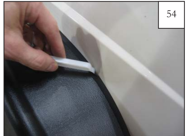
Use the hooked end of the edge trim tool to check for full adhesion. Do this by sliding it along the top of the edge trim to visually verify that the tape is adhered to the vehicle surface. Repeat step 51 if tape is not fully adhered to the vehicle surface.
