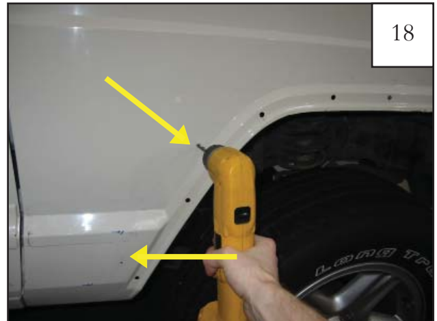
Remove inner piece from front fender. Using a 1/4" drill bit, drill through sheet metal on locations marked in previous step. Pre-drill with a smaller drill bit if desired.
