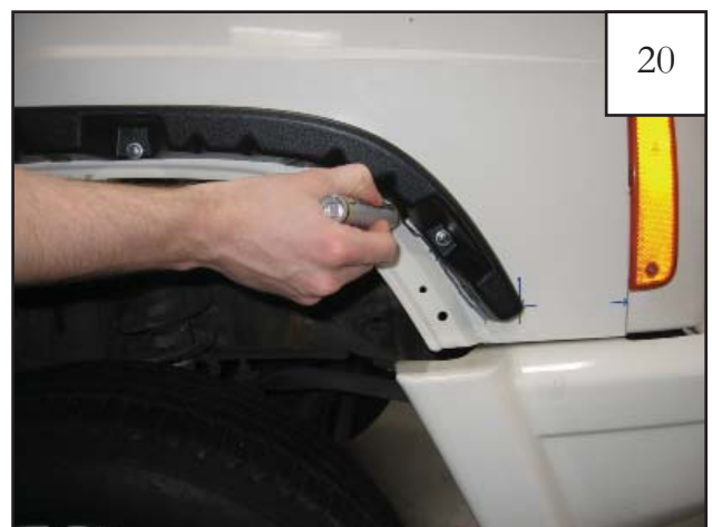
Using a grease pencil or marker, use the inner profile of the installed inner pieces as a guide to mark the sheet metal for trimming.
