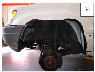
Completed cut-out with caulking applied.
