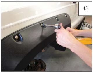
Hold flare in place on fender. Using the provided torx bit driver and ratchet with 3" extension, start each screw into drilled holes.
