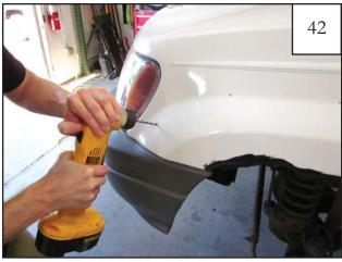
Using a 3/16" drill bit, drill holes marked in step 41.
