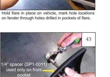
Install a Torx screw (SW1-0045) through **FRONT** pocket hole of flare and secure with rubber spacer **(SP1-0011)** using supplied #45 Torx bit (SW1-0052). The torx bit fits into a 5/16" socket. Use with a 3-6" extension for drill or air ratchet. Drive screw into spacer until tight.
