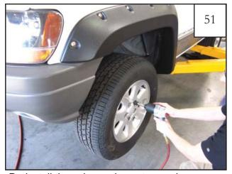
Re-install tire using an impact wrench.
