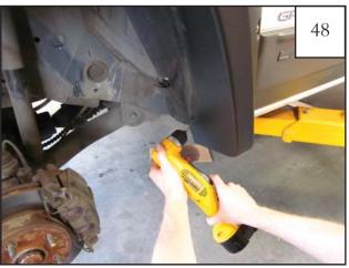
Using a 3/32" drill bit, drill hole through flare into sheet metal near the back inside edge of the wheel well.
