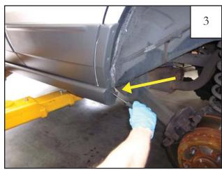
(Note: For models with Rocker Panels installed) Using a #2 Phillips Screwcriver, remove screw from rocker panel in rear wheel well.
