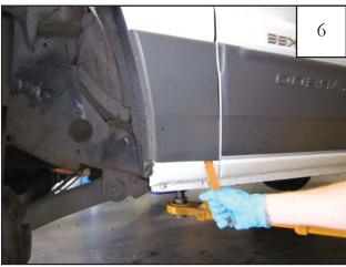
Using a pry tool, separate the factory front side cladding from the sheet metal along the bottom taped edge.
