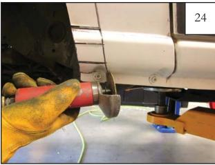
Using cut off wheel remove section containing bolt at the bottom pinch weld of fender. See step 25 for illustration of section to be removed.
