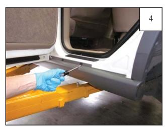
(Note: For models with Rocker Panels installed) Open front and rear doors. Using a pry tool, remove retainers along top of rocker panel.
