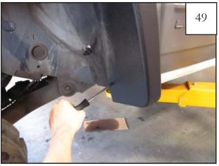
Using a philips screwdriver, install supplied screw (SW1-0056) into hole drilled in step 47.
