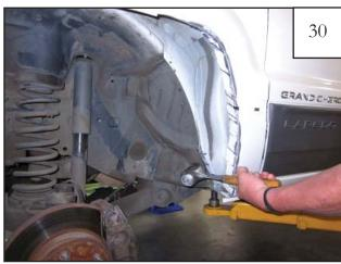
Using a hammer, pound the tabs made in the inner pinch weld flat against wheel well.
