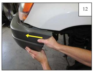
Push front bumper forward away from wheel well to release from factory installed clip in fender.
