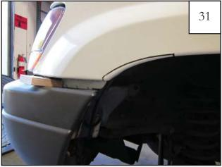
Use a small wood block to prop the bumper away from the fender in preperation for sheet metal trimming.
