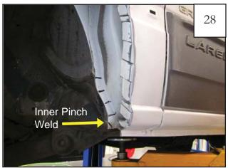
Mark the inner pinch weld with 5 lines appoximately 2 inches apart starting from the bottom.
