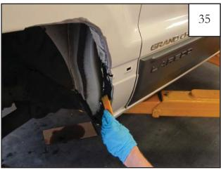
Apply urethane caulking or primer to seal any exposed sheet metal for rust prevention.
