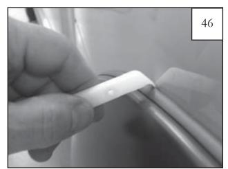
Using supplied Edge Trim Tool (ET1-0002), seat edge trim against vehicle by hooking curved end under edge trim at one end of flare. Next, slide around outer edge of flare to the other end. You should repeat this process once screws are tightened.
