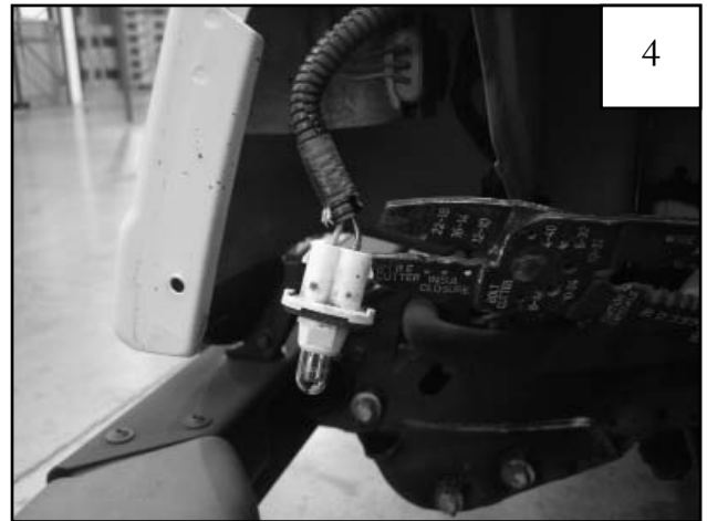
4 Use wire cutters to cut the two wires at the base of the factory side marker lamp.
