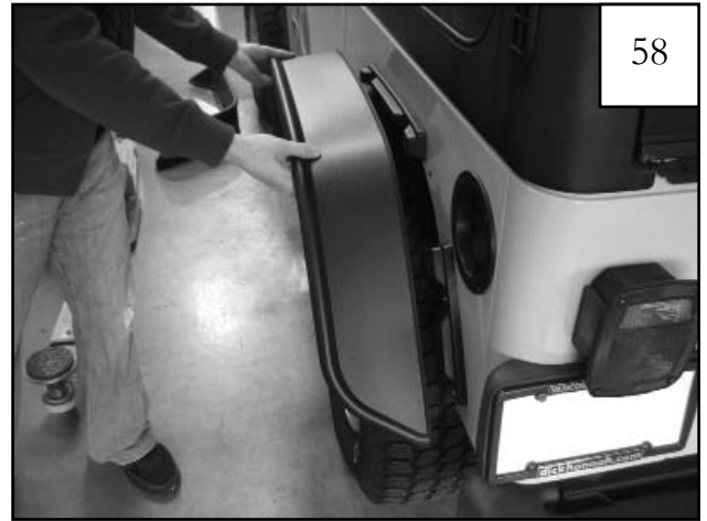
Place the outer flare over the inner pieces and push until snug against the vehicle surface.
