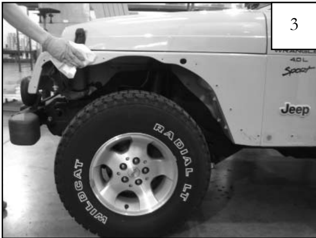
3 Remove the factory installed fender flares. Thoroughly clean the exposed metal fender with a damp cloth and dry.
