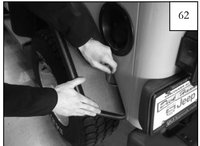
Peel outer tape liner from the double-taped edge trim. Push down lightly on the fender flare to create a small gap between the sheet metal and the edge trim. This makes it easier to pull the red liner.
