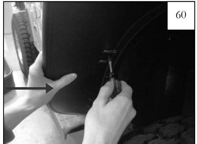
Hold flare in place on fender and start a #8 pan head screw (SW1-0056) into each hole location and through the speed clip (CL1-0022) on inner structure (6 locations). Do not tighten.
