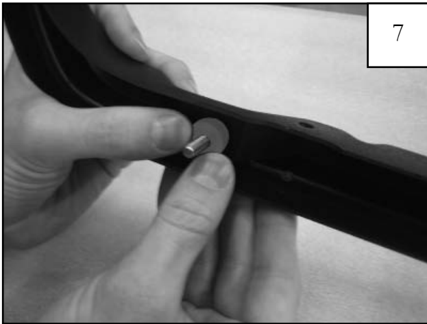
7 Push the rubber spacer (SP1-0011) and machine screw (SW1-0053) together until they are both tight against the inner piece. Spacer has been lightened in picture for visibility.
