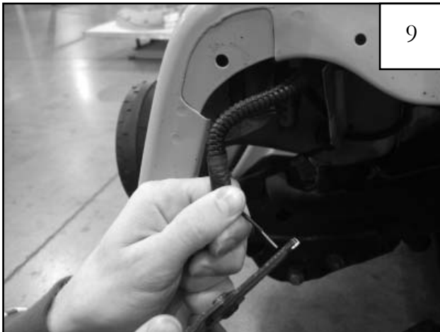
9 Use wire strippers to strip away approximately 3/8" of wire covering from the factory installed side marker lamp wires.
