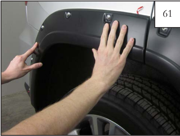
61 Hold Rear Main Flare up to wheel well to confirm fit. Do not install fasteners at this time.
