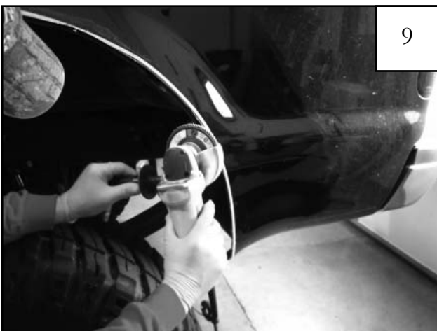
Using a grinder, deburr cut edges.
