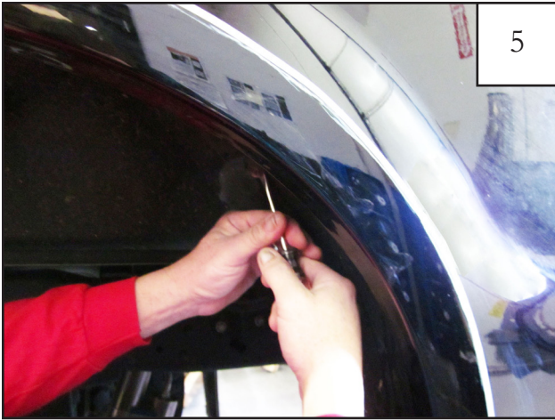
Using a pry tool, remove two factory installed tuflocs from splash guard
