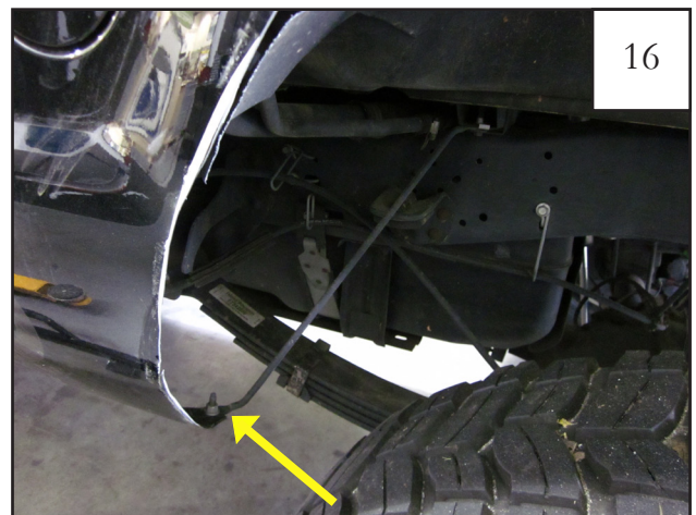
Remove factory support bar bolt, and save for reinstallation.
