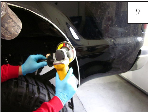
Using a grinder, deburr cut edges. Treat any bare sheet metal with rust resistant paint BEFORE continuing.
