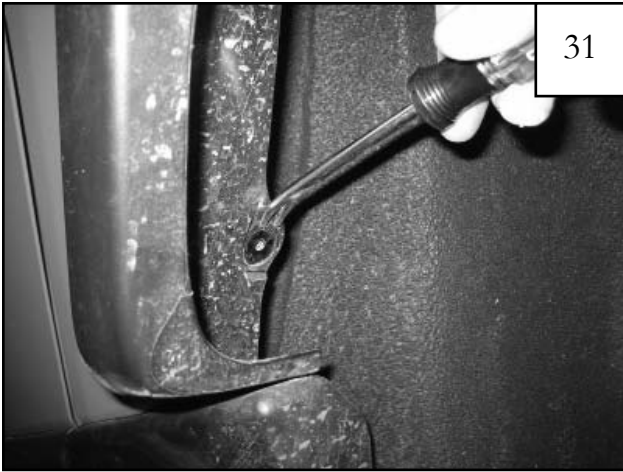
At front of wheel well, use pry tool or knife to pry plastic grommet from sheet metal. Discard grommet, leaving a square hole.
