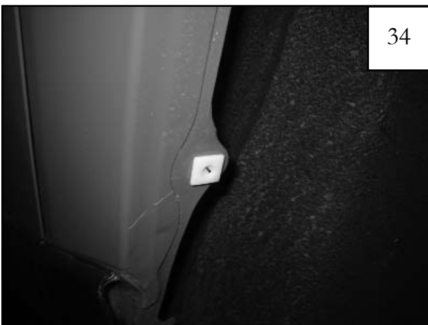
Install a supplied Grommet (GR1-0002) in square hole at front of wheel well.
