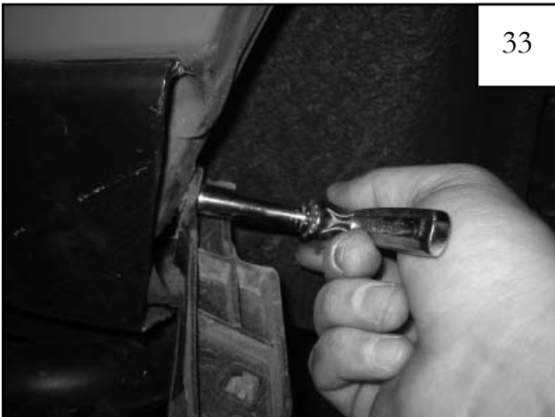
Remove last bolt holding the rear flare on, at the front of the wheel well. Remove flare.
