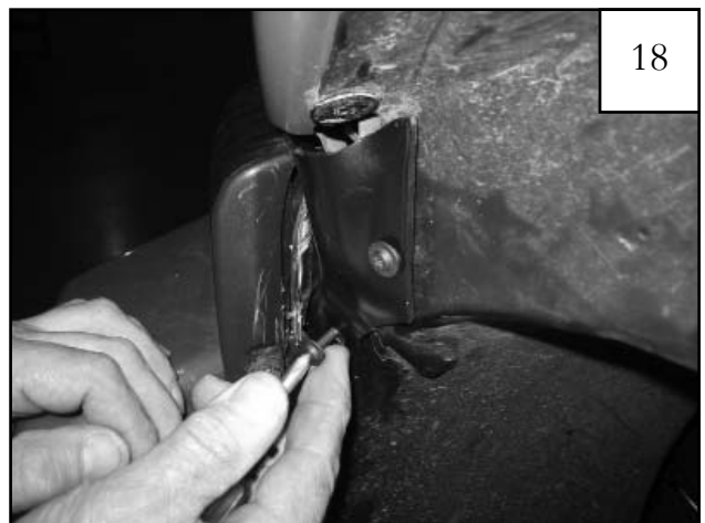
Position Inner Front Piece on vehicle, aligning holes in part with holes in Clips installed in previous Step. Install supplied Screws (SW1-0056).
