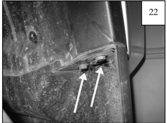
Remove two bolts from mud flap.
