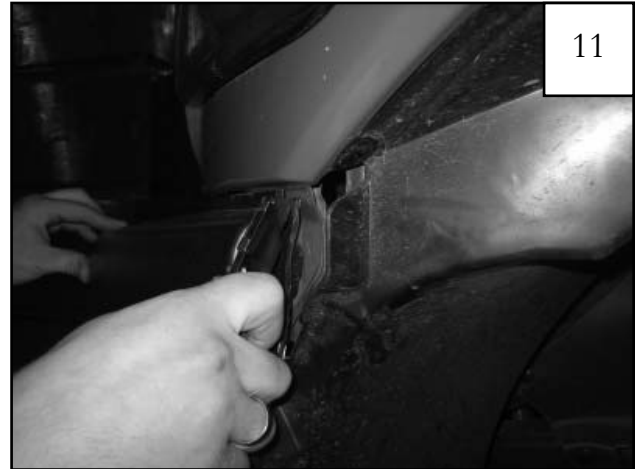
Trim remaining plastic flush with bumper.
