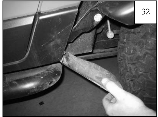
Cut along rocker panel so that it is trimmed flush with sheet metal.
