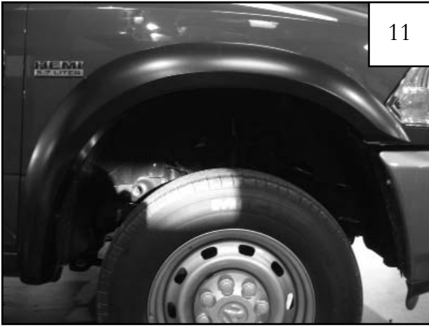
Completed front flare installation.
