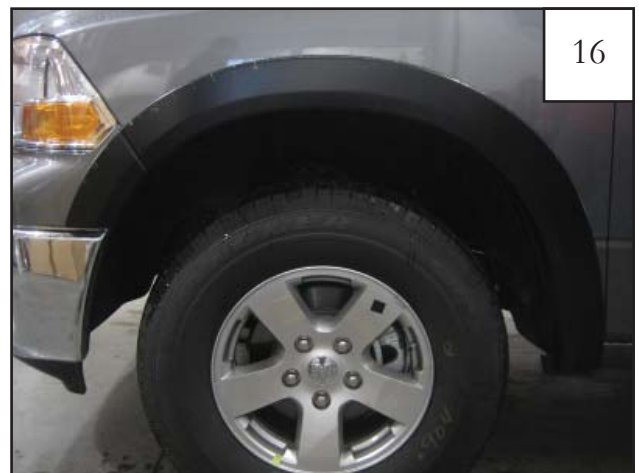
METAL BUMPER ONLY: Completed front flare installation.
