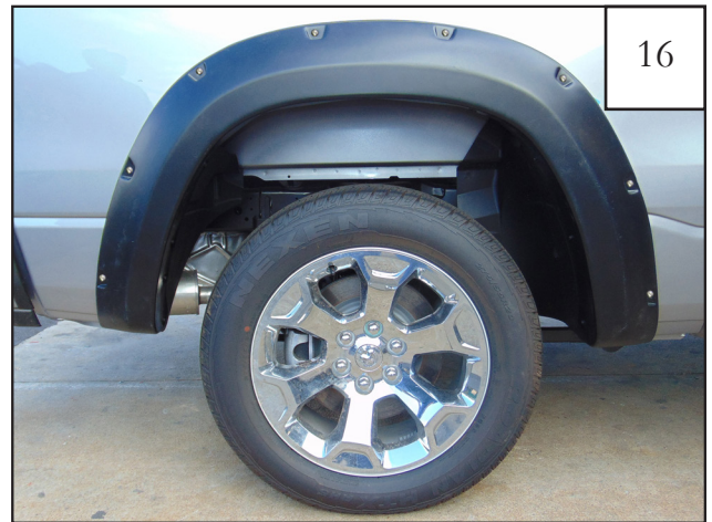
Completed rear flare installation.
